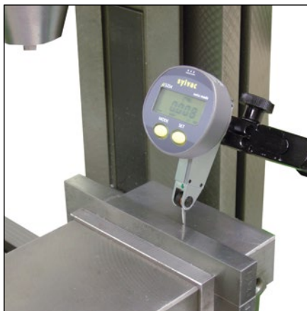
Checking the alignment on milling machine.
